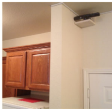
(a) Single Kinect setup for fall prevention in elderly residence [1]
